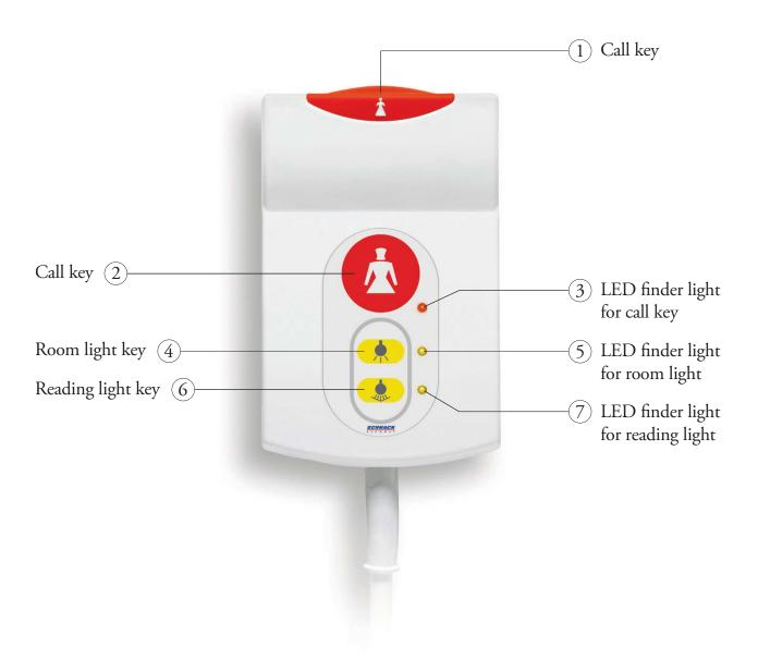
CAUTION: It must be checked that the device is fully functional each time the device is plugged in and each time a disconnection call is reset. Please note that a disconnection call is automatically triggered when the device is unplugged.
